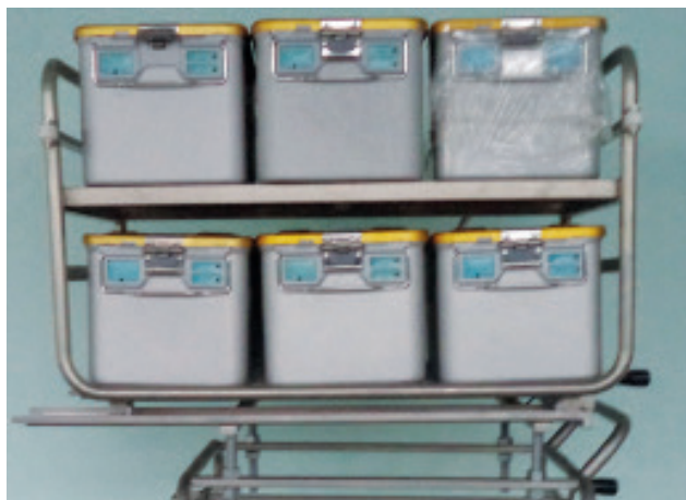
Manual loading of containers or various packs using a loading platform and loading module on a loading trolley. Also using optional loading module(s) to process containers
